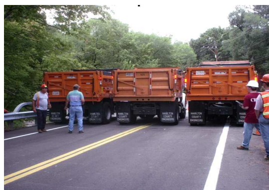
FIGURE 2 TRUCK ON THE BRIDGE DECK FOR TESTING
