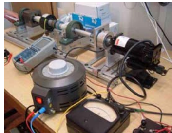
THE SLIP-RINGS TEST BED
