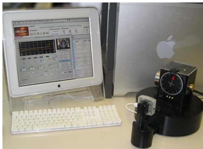
FIGURE 2 THE REMOTE LAB ELECTRICAL DRIVE SETUP.
