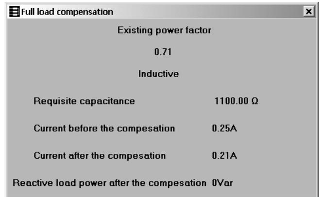
FIGURE 6 FULL REACTIVE LOAD POWER COMPENSATION WINDOW.
