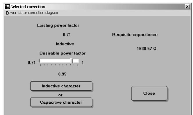
FIGURE 7 WINDOW FOR SELECTED POWER FACTOR CORRECTION.
