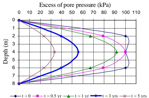
FIGURE 2 RESULTS OF EXCESS PORE PRESSURES ON EXCEL
