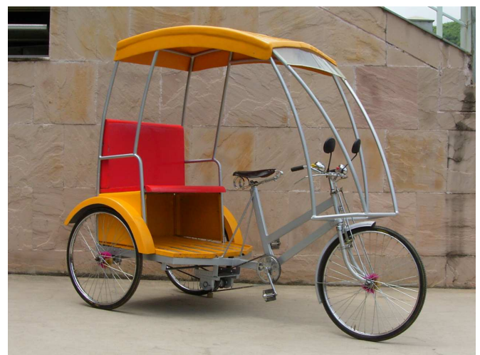
FIGURE 2 DIPBAHAN-A TRICYCLE RICKSHAW DESIGNED AND PROTOTYPED.
