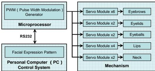
Figure 2 Architecture of an Affective Robot
