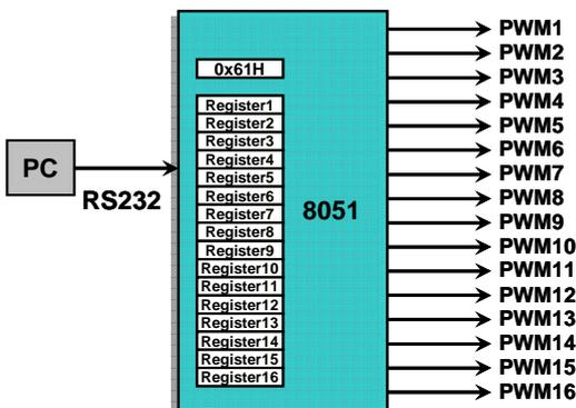
Figure 4. Architecture of the Micro Controller
