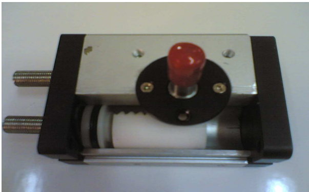
FIGURE 13 A TYPICAL SAMPLE OF CUT-AWAY SECTIONS (ROTARY ACTUATOR)
