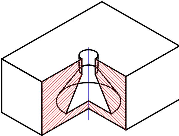
FIGURE 1 IMPOSSIBLE TO MAKE - WHOLE OF CONIC SHAPE
