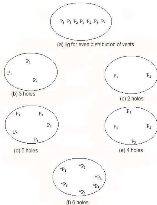
FIGURE 1 PREPARATION AND CONFIGURATION OF JIGS SHOWING THE LAYOUT USED FOR EVENLY DISTRIBUTED VENTS (A) AND FOR THE 2 – 6 HOLES SHOWN IN (B), (C), (D), (E) AND (F).
