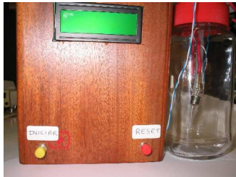
FIGURE 1. DSP UNIT AND TEST CHAMBER WITH S_xO_2 SENSORS.
