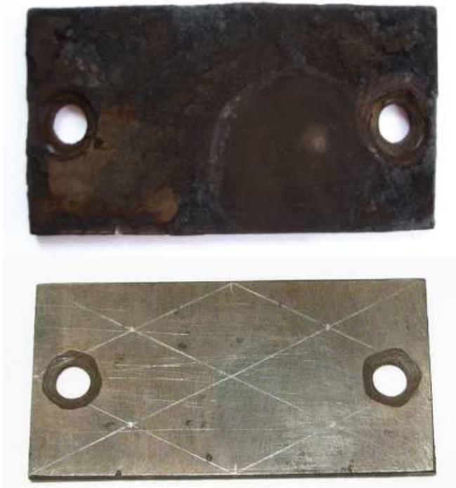
FIG.2 PHOTO OF A CONTROL PLATE. AS IT WAS REMOVED FROM A BOILER (TOP) AND AFTER CLEANING (DOWN). ON THE BOTTOM PLATE VISIBLE LINES WHICH INDICATE MEASURING POINTS. REAL SIZE 100X50 MM [1]
