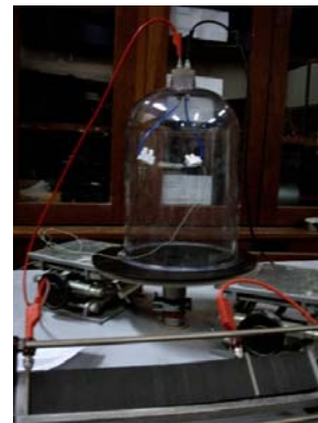
FIGURE 3 APPARATUS FOR STUDYING COOLING BY CONVECTION AND RADIATION.
